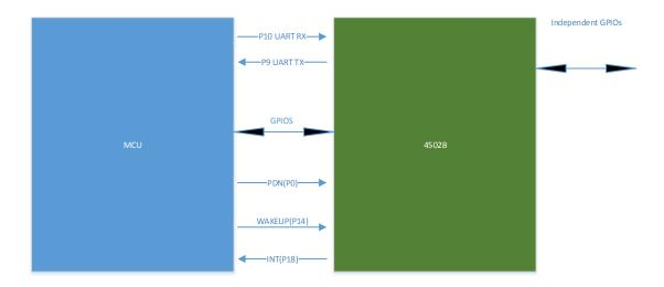
Figure 1.Application Schematic of the Pass-through Module
